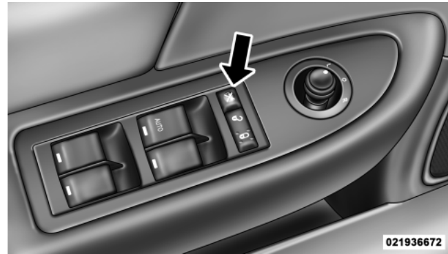
Window Lockout Switch
