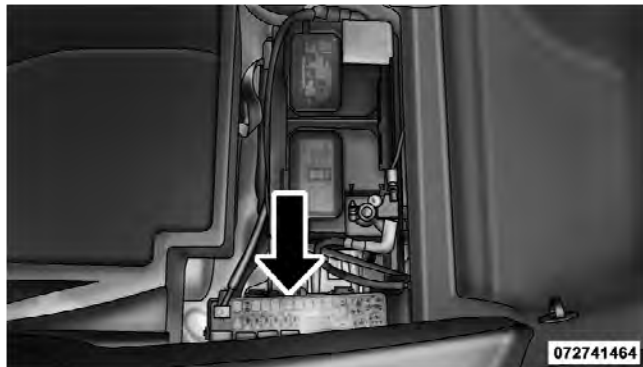
Rear Power Distribution Center
