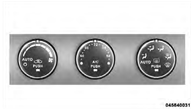
Automatic Temperature Control
