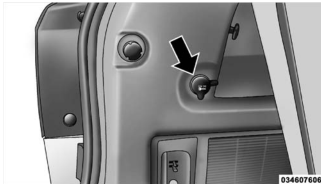
Rear Power Outlet
