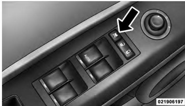
Window Lockout Switch
