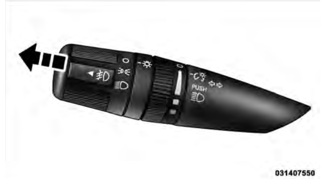
Front Fog Light Control
